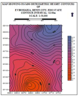
Fig. 7: EGM96 Derived Orthometric Heights
