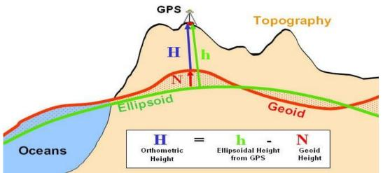
Fig. 1: Relationship between orthometric, geoid and ellipsoidal heights
